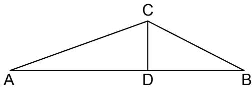
Figure 2: Schematic of the points of interest in the intersections of two spheres. A and B are the sphere centers, C is on the intersecting circle, and D is the center of that circle. The circle itself is perpendicular to the page.
